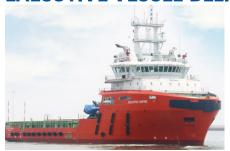
The Colombo Dockyard in Sri Lanka has delivered newbuild AHTS vessel Executive Aspire to Executive Offshore. Following delivery, the vessel has since been mobilised to Singapore. The Executive Aspire was built to a Wärtsilä design, with a length of 78.2m and a breadth of 18.5m. She has a bollard pull of 200t and a deck area of 600m², with a deadweight of around 3,000t and an accommodation capacity for 44 persons.
