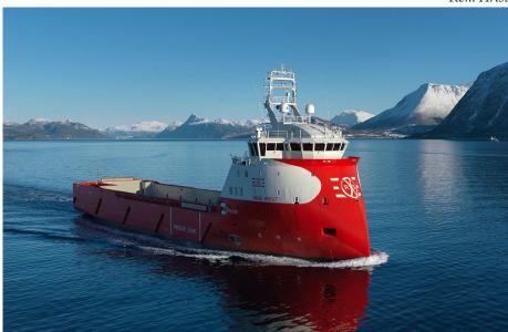
delivered in 2011, were built to the Ulstein PX 105 design. The Rem Eir has a length of 92.5m and deck area of 1,090m², while the Hrist and Mist have a length of 88.8m and deck area of 916m². In addition to the Rem Eir, Hrist and Mist, Remøy Shipping is also the owner of one seismic vessel and one coastguard vessel, while also managing a wider fleet of externally owned vessels.
