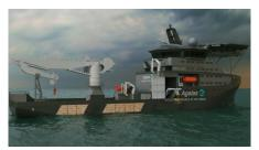
Newly formed Norwegian vessel owner Agalas has bucked the trend and become the first owner to order a newbuild CSV in more than seven years. The 99.9m CSV will utilise methanol dual fuel and battery propulsion to reduce emissions by as much as 70%. The Sefine Shipyard in Turkey will build the vessel, which will be equipped with a 150-tonne AHC crane, dedicated ROV hangars, a helideck and 1,000m² of deck space, with accommodation
